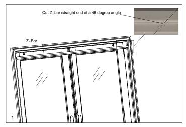
NOTE: Z-bar location is next to the part stop on 69/16  $^{\prime\prime}$  (167) and 49/16  $^{\prime\prime}$  (126) jamb units.
