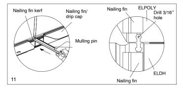
5. Apply a third clamp and wood blocks to interior as needed. Make sure mulled units are flush and square at the sill and jamb liners. Fasten interior of mulled units with 1/2" x 1" 16 gauge staples spaced every 4" (102). See illustration 11. Fasten the jambs at each end with steel mullion ties and two #7 x 5/8" Phillips flat head wood screws into each unit. See illustration 12.
