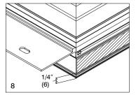
head jamb of the lower unit. Mull tape should be located 1/4'' (6) from the exterior edge of the Ultrex frame. See illustration 8.
