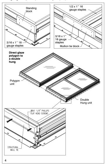
7. Install a steel mullion tie across the head jambs and fasten with two #7 x 5/8" Phillips flat head wood screws into each unit. See illustration 5. If mulling a direct glaze polygon to a double hung unit, attach steel mull tie to the sills as well as the head jambs.
