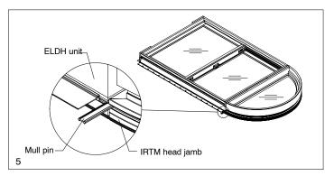
Lightly clamp units together at the ends of the mullion. Fasten interior of mulled units with 1/2" x 1" 16 gauge staples 1" from edge of jamb and spaced every 4" (102). See illustration 6.
