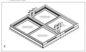
Slide the mulling pin in the full length of the mullion. A hammer may aid in the application of the mull pin. The mull pin ends must be recessed 1/4"(6) to allow sealant application later. See illustration 3.
