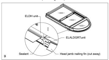
Seal around the edge of the connectors as shown in illustration 10. If applicable, jamb extension can now be installed. Follow installation instructions for installing unit into rough or masonry opening.
