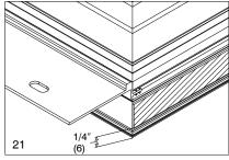
Apply mull sealing tape along the full length of one jamb to be mulled ensuring it is located 1/4'' (6) from the exterior edge of the Ultrex frame as shown in illustration 21.
