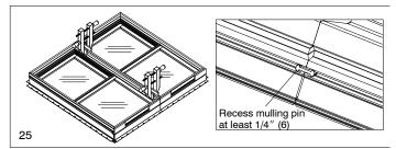
7. Apply a third clamp and wood blocks to interior as needed. Make sure mulled units are flush and square at the sill and jamb liners. Fasten interior of mulled units with 1/2" x 1" 16 gauge staples spaced every 4" (102). Remove the wood standing blocks at the sills near the mullion. Replace with a wood mullion tie block (W8952) and attach with 3/16" x 1"18 gauge staples. See illustration 26.
