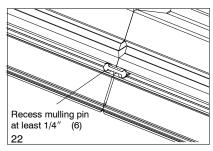
1/4" (6) on each end to allow for sealant placement and horizontal mulling pin application later. See illustration 22.
