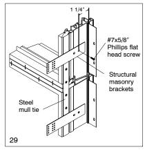
NOTE: Interior mull trim should be applied after unit is completely installed and interior trim is applied
