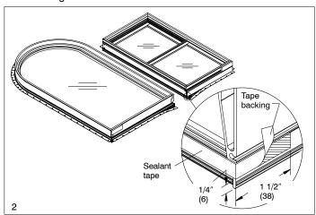
Partially pull nailing fin/drip cap from sills at mullion to expose side jamb nailing fin kerf and allow for mulling pin installation later.
