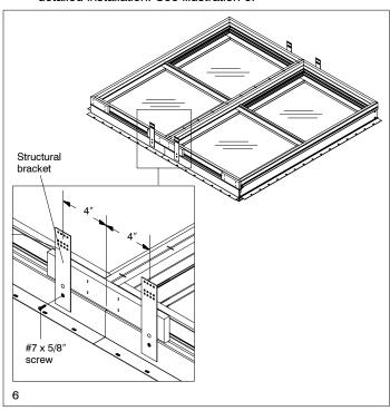
9. Apply silicone sealant at the mullion from the frame exterior edge to the drip cap/nailing fin kerf and across the kerf over the mulling pin as shown in illustration 6. Apply nailing fin connector at the head jamb and sill by removing the paper backing from the connector and pressing into place. See illustration 7.
