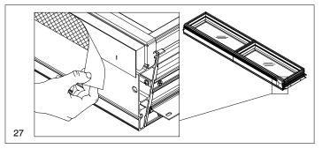
Apply a third clamp and wood blocks to interior as needed. Make sure mulled assemblies are flush and square at the sill and jamb liners. Fasten interior of mulled assemblies with 1/2" x 1" 16 gauge staples spaced every 4" (102). See illustration 28.
