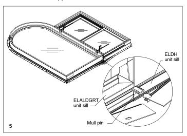
7. Join the wood frame members along the interior of the mullion. Apply additional clamps as needed. Make sure mulled units are flush and square at the sill and jamb liners. Fasten with 1/2" x 1" 16 gauge staples spaced every 4" (102). Center the mull splice block over the mullion at the sill and attach with 3/16" x 1" 18 gauge staples. See illustration 6.
