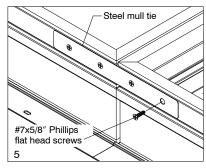
Install structural brackets 4" (102) from the mull on both sides. Attach each of the brackets with the #7 x 5/8 screws provided. Follow the instructions provided with the brackets for more detailed installation. See illustration 6.
