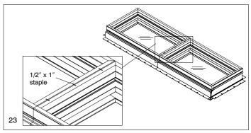
4. Remove paper backing from adhesive tape on one side of structural mull tie and carefully install on sill of upper two wide assembly. Do not remove paper backing from tape on bottom side of mull reinforcement at this time. Attach reinforcement to wood sill liner with 3/16" x 1" 18 gauge staples spaced every 6" (152). Carefully set upper unit aside. See illustration 24.
