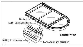
NOTE: It is important that care be exercised when moving a mulled assembly from the mullion area to the rough opening. Interior mull trim should be applied after unit is completely installed and interior trim is applied.
