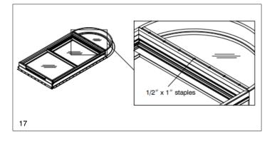
6. Center mulling tin over mullion 3/8" (10) from interior and fasten to ELALDGRT unit and wood jamb liner of ELDH unit with 1/2"x1/2" staples following the pattern shown in illustration 18. Fold the jamb nailing fin over the mulling tin and mark a line with a pencil as shown. Using the pencil line as a reference, pre-drill at screw locations indicated with a 7/64" drill bit through the first layer of the double hung Ultrex jamb as shown. Fasten with 3/8" pan head screws.
