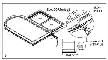
Position the units together in the desired configuration. Check to be sure that frames at both ends of the mullion are flush and the nailing fin kerfs are aligned. Lightly clamp units together on interior near each end to hold two mulled units in place. See illustration 4.
