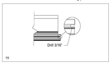
Align round top flush with side jambs and exterior of the double hung unit, align and press barb into double hung head jamb drip cap kerf to mull.
