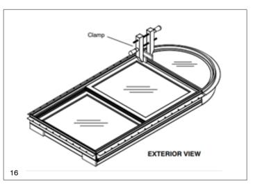
Lightly clamp units together on interior (use wood blocks to protect interior near each end to hold two mulled units in place. Fasten interior of mulled units with 1/2" x 1" 16 gauge staples spaced every 4" (102). See illustration 17.
