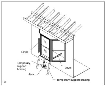
12. Center unit in the opening with approximately 1/2" space on each side of the unit. Plumb and square the unit with the aid of a level and jack, ensure the interior jamb extension is flush with the interior wall and temporarily fasten the headboard to the header with three #8 x 3" flat head screws. See Illustration 10.
