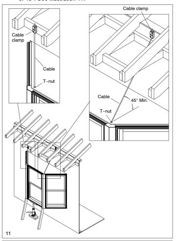
**Hint:** The cables can be angled inwards to fit under the unit roof to allow a steeper cable angle.
