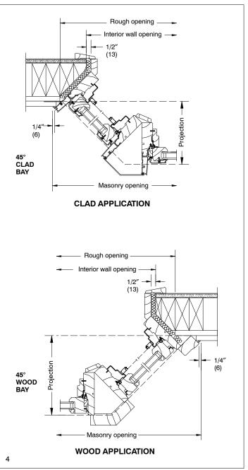
5. For frame construction, the support platform of the Bow or Bay must follow the radius or the angle of the particular Bow or Bay unit and be located directly under the sill or subsill. The support platform should be level, however, the sill/subsills can be shimmed to bring the unit level after placing in the rough opening. See illustration 5.
