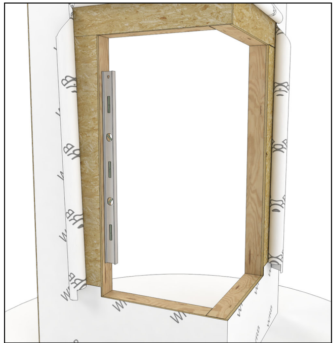
Figure 12 Check the jambs for plumb
