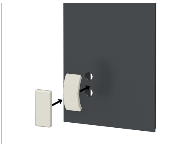
Figure 90 Flex the bumper and insert in bottom of jamb cover
