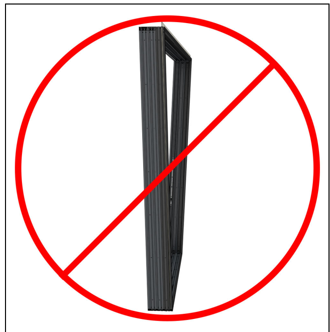
Figure 62 Make sure the entire frame is on the same plane and not twisted.
