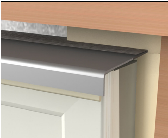
Figure 23 Apply sealant between window and exterior finish.
