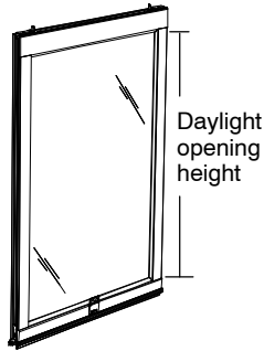
Top Sash Interior View
