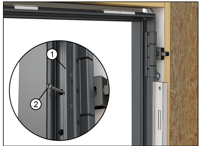
Figure 41 Plumb interior to exterior, shim and fasten
