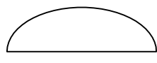
Half Ellipse Made using two or more radii. Also called compound radii ellipse. Not true radius.
