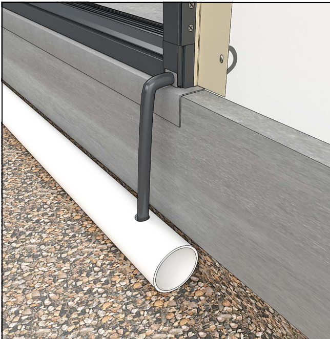
Figure 9 Weep tube terminating into drainage pipe
