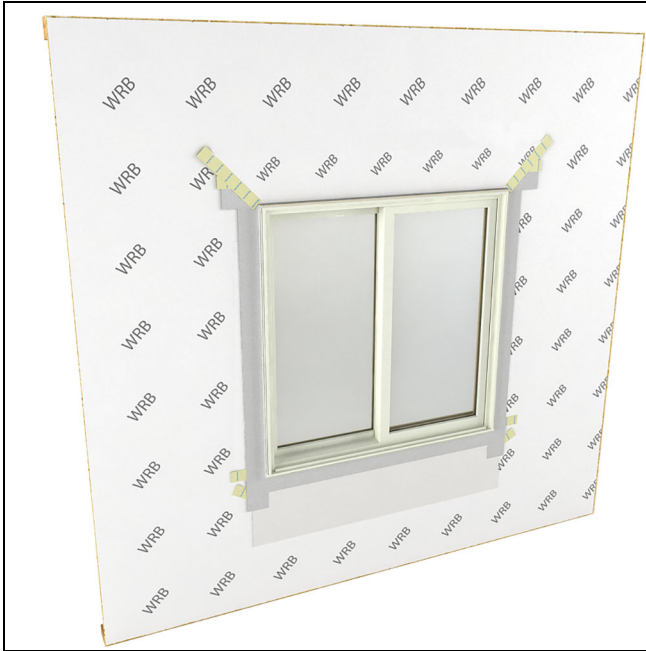
Figure 19 Sealing the Installation in air barrier applications.
