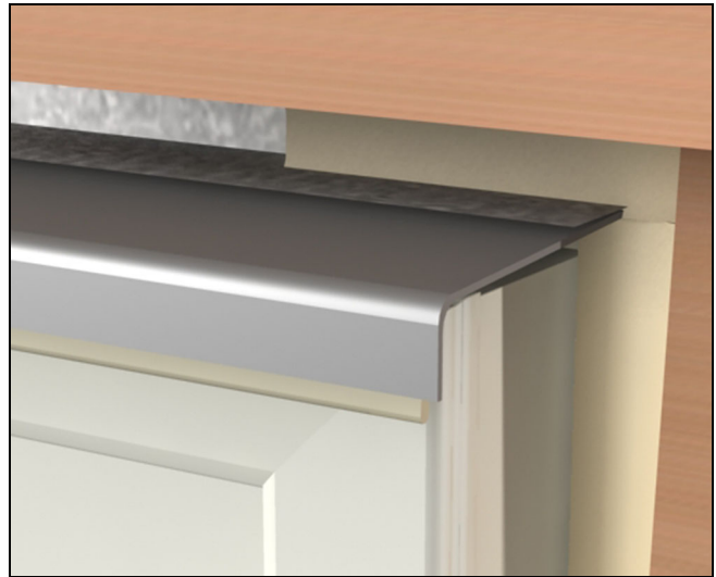
Figure 23 Apply sealant between window and exterior finish.
