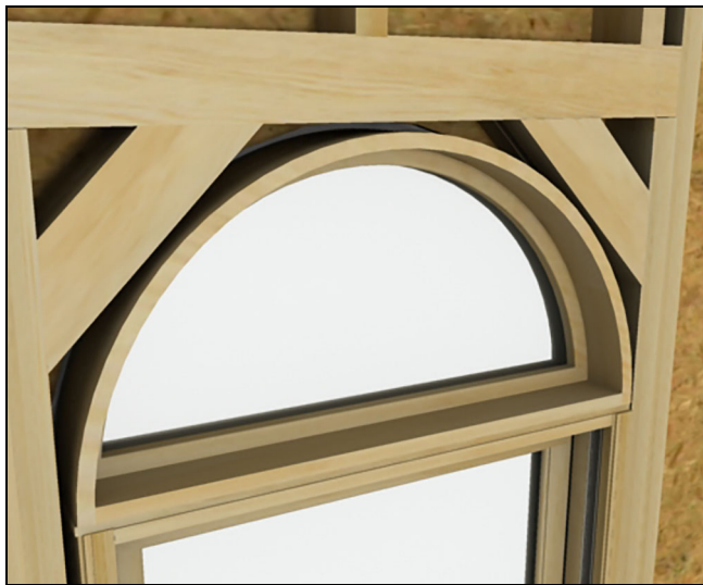
Figure 3 Typical rough opening.
