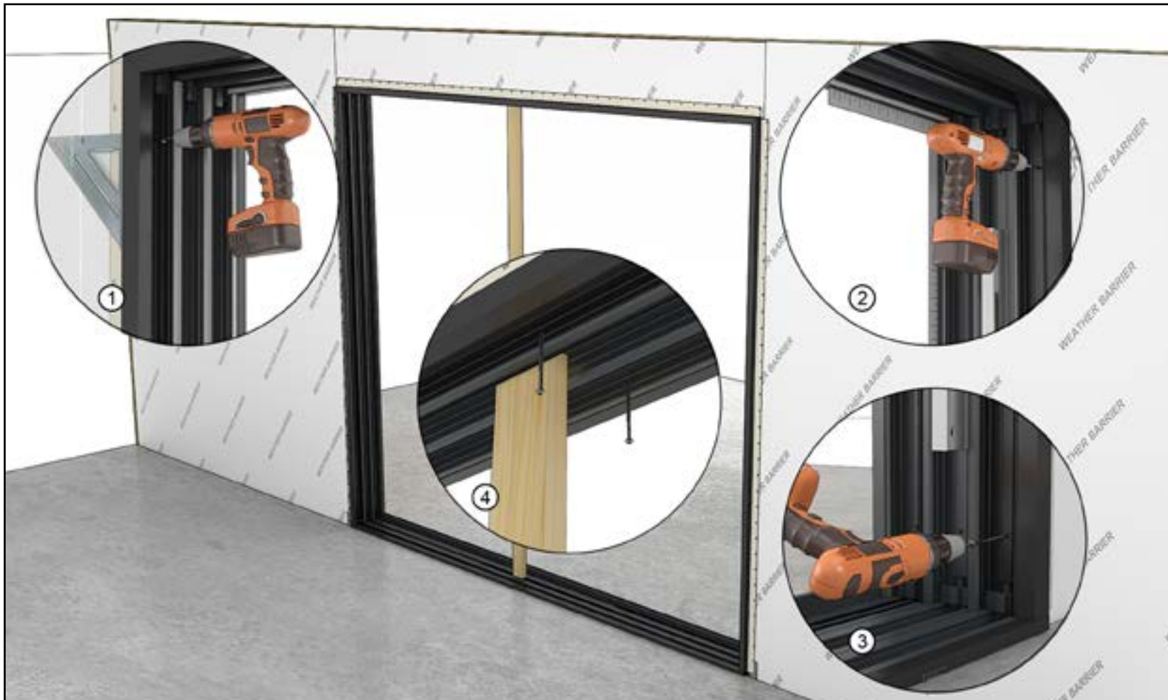
STEP 7 SQUARE THE FRAME AND COMPLETE FASTENING
