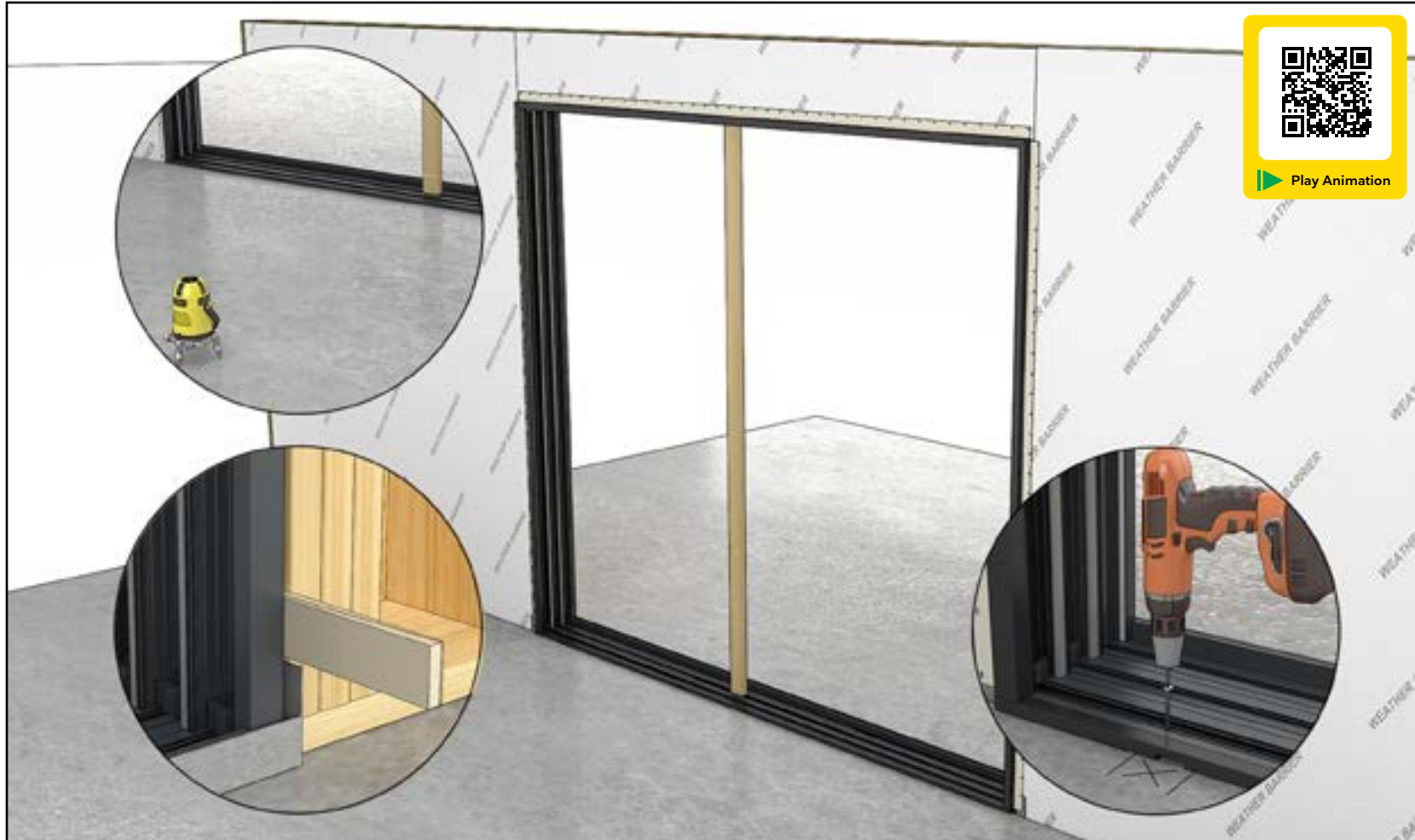
STEP 6 INSTALL THE FRAME: Center the frame in the opening. Verify the sill is level. Shim the bottom of the jamb and fasten the sill near the stationary side.
