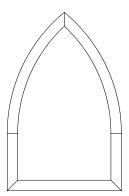
Any unit with a continuous springline will need to be spliced at the point of springline unless specified on order.
