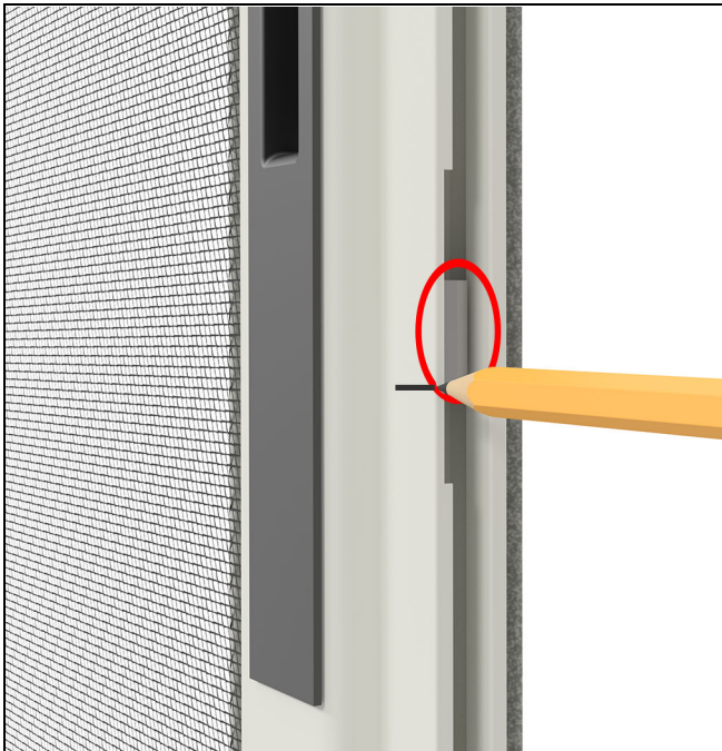
Figure 4 Make a mark even with the bottom of the latch
