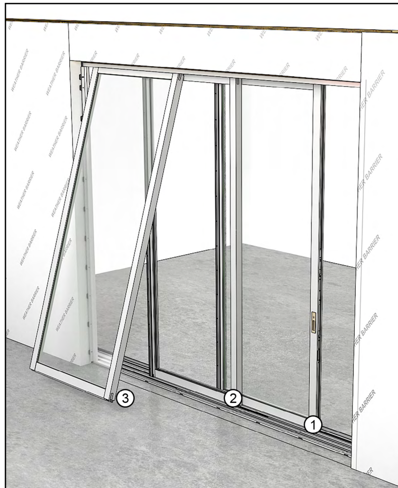
STEP 10 INSTALL the secondary panel(s) (2) overlapping the primary (1) and then the pocket panel (3) last.
