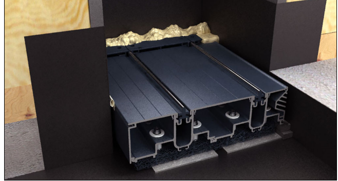
Figure 4 Pocket with open face slot in concrete with a 2 3/8" (60) slot recess leaving 0" available floor thickness. The concrete is the finished floor and flush with the top of the sill.
