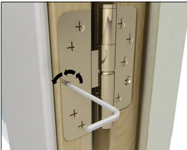
Figure 32 Counterclockwise to move panel away from jamb.
