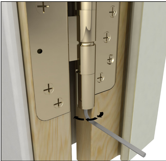
Figure 35 Lower the panel, counter-clockwise adjustment
