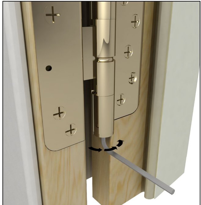
Figure 34 Raise the panel, clockwise adjustment
