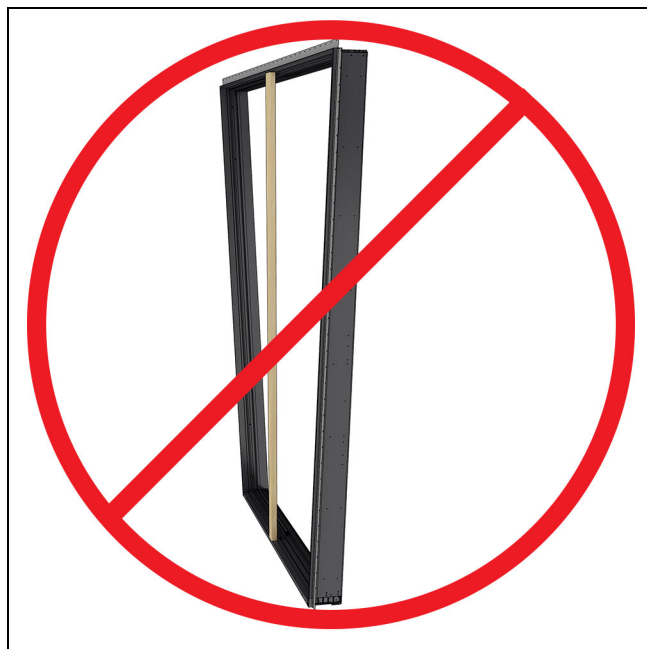
Figure 50 Make sure the entire frame is on the same plane and not twisted.
