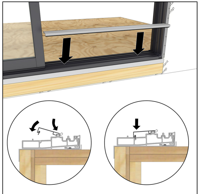
Figure 78 detail of sill cover
